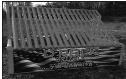
LR8 model , skid steers-mini excavators, Adjustable bar and cleaner option available, AB set up at 2"-adjustable in 1" increments
